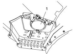
The drain screw is located at the bottom of the recoil housing. Use a wrench to remove the screw. Be sure to reinstall the screw after draining the housing.
